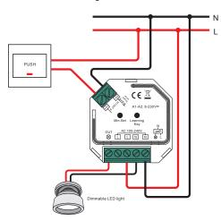
This phase dimmer adopts trailing edge dimming (reverse phase control), please make sure the connected loads support alternating current. Please refer to the user manual of the load or consult the supplier of the load.
