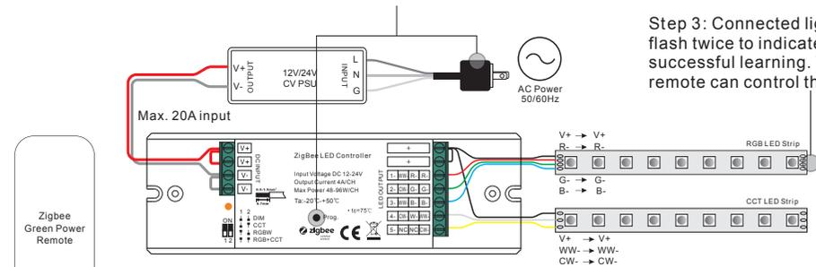
Step 3: Connected light will flash twice to indicate successful learning. Then the remote can control the device.
