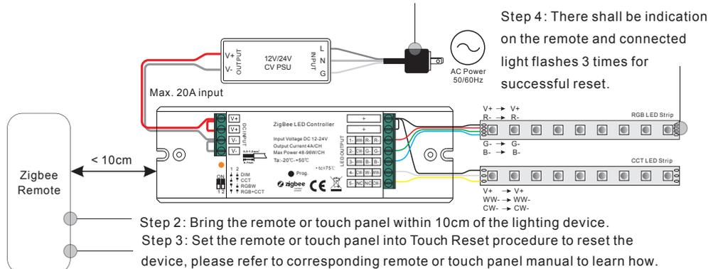
Step 4: There shall be indication on the remote and connected light flashes 3 times for successful reset.
