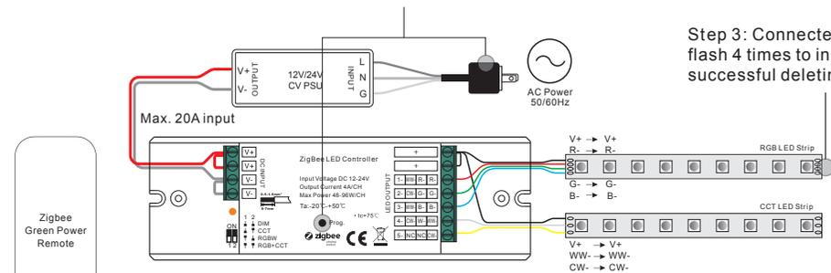
Step 3: Connected light will flash 4 times to indicate successful deleting.
